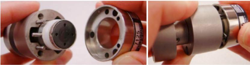
9. Remove the stator face assembly from the stator and replace with the new one. (For SFAs with 2 pins, it can be put in either way. For SFAs with three pins it can only be inserted in the correct direction.)
