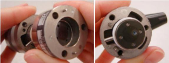
4. Remove the rotor seal.
