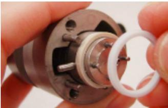
6. Put in the new isolation seal. The open side faces the bearing ring. (toward the handle end)
