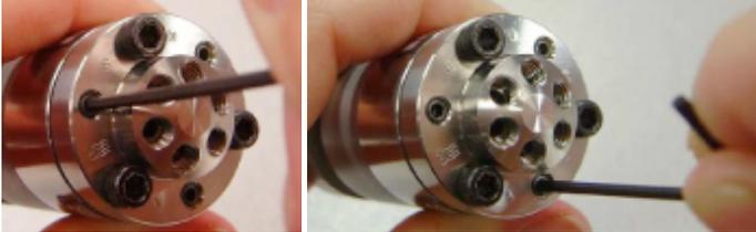
12. Tighten each stator screw a little at a time (1/8 turn or less, working your way around the valve) until the leaking stops. Double check that the gap between the stator and stator ring is the same all the way around. Retighten the set screws so that they touch the stator ring.
