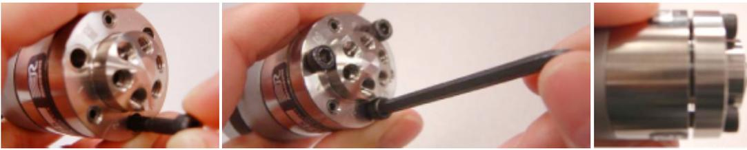
Reattach the valve to your system. Test the valve to see if it holds pressure. If the valve leaks you will need to tighten the valve. First loosen the set screws the same amount for each one.
