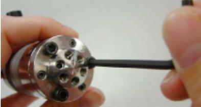
13. Remove the needle guide in the handle. (Use pliers if necessary.) You can do this with the handle removed if you prefer. (To remove the handle, loosen the 2 set screws.
