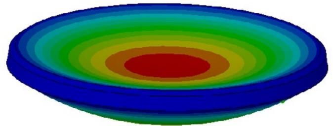
**Figure 11 : FEA prediction of self-weight distortion of the same lens element resting on a perfectly circular seat. The resulting distortion is approximately seven times smaller.**
