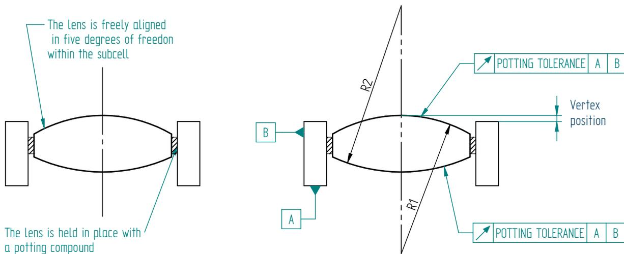
**Figure 7: Gap potting with high precision active lens alignment.** The element is freely positioned relative to the OD and one side of the subcell so that both centers of curvature are aligned. The flange distance is also precisely controlled. Lens wedge and diameter do not affect element placement accuracy. Only high precision is needed on the form tolerances of the subcell's reference surfaces (i.e. parallelism, roundness, and flatness).
