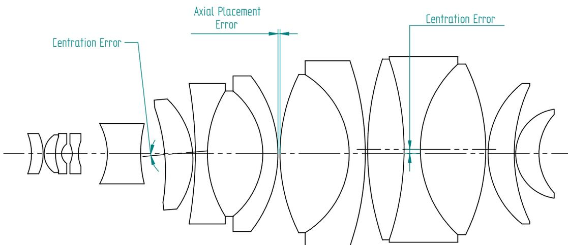
Figure 1: Multielement lens assembly with incorrect element placement: the optical axes of the elements do not coincide with the axis of the barrel and the airspaces are not correct.
