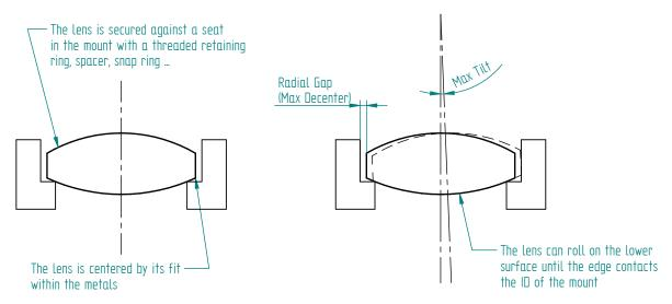
Figure 3: Drop-in or edge-mounted construction: the element can roll and is aligned by its fit within the metals. Lens wedge and diameter affect element placement accuracy.
