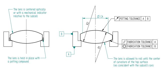
Figure 4 : Active element alignment. The lens element is actively centered within its subcell and potted in place. Lens wedge and diameter do not affect element placement accuracy.
