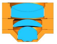
Figure 8 : Melles Griot Exact Placement with the barrel-less construction (bottom) versus the traditional cell-mounted construction (top).
