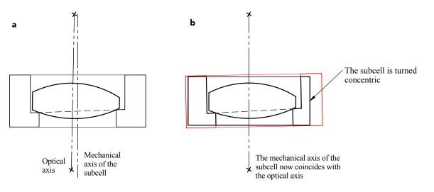
Figure 5: Mounted element centering a) the optical axis of the mounted lens is determined, b) the subcell is trimmed to final size with its outer diameter aligned parallel to the optical axis.
