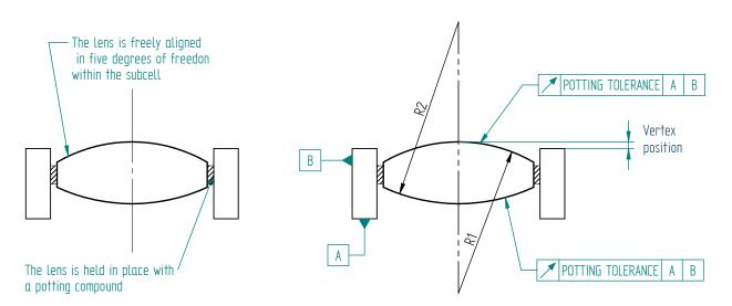
Figure 7: Gap potting with high precision active lens alignment. The element is freely positioned relative to the OD and one side of the subcell so that both centers of curvature are aligned. The flange distance is also precisely controlled. Lens wedge and diameter do not affect element placement accuracy. Only high precision is needed on the form tolerances of the subcell's reference surfaces (i.e. parallelism, roundness, and flatness).
