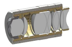
Figure 6 : Example of stacked-cell assembly using the mounted element centering method. The opto-mechanical configuration and subcells' design were specifically adapted to use CNC-controlled turning for the machining and alignment of the cell-mounted lenses.
