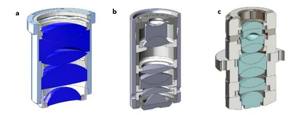
Figure 2: Melles Griot Exact Placement assembly technology enables a much higher level of positioning accuracy than the drop-in and conventional cell-mounted construction methods. \* "Centration Error" is measured as a surface-normal TIR (Total Indicated Runout) at the edge of the clear aperture
