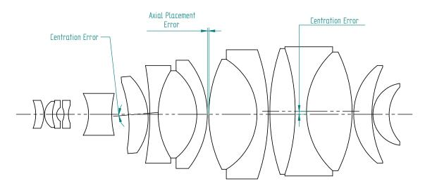
Figure 1: Multielement lens assembly with incorrect element placement: the optical axes of the elements do not coincide with the axis of the barrel and the airspaces are not correct.
