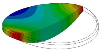
Figure 10 : FEA prediction of a meniscus lens resting in a subcell with primarily two-point contact. The upward facing concave surface exhibits a strong distortion with an astigmatic saddle shape.
