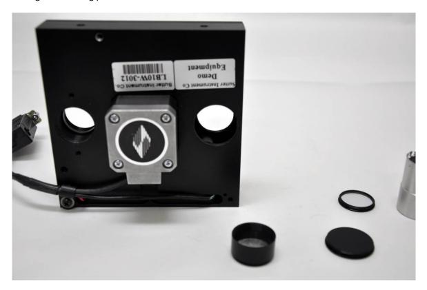
4. Orient the new filter wrench vertically and install the threaded filter on the wrench. The design of the filter wrench should allow some flexibility to secure the threaded filter in place.
