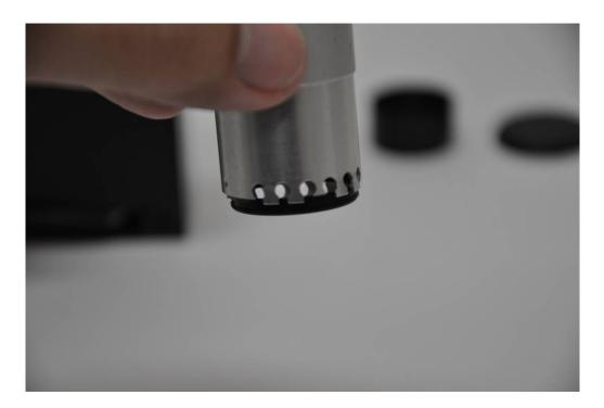
5. With the threaded filter secured to the wrench, thread the filter directly into the filter wheel.
