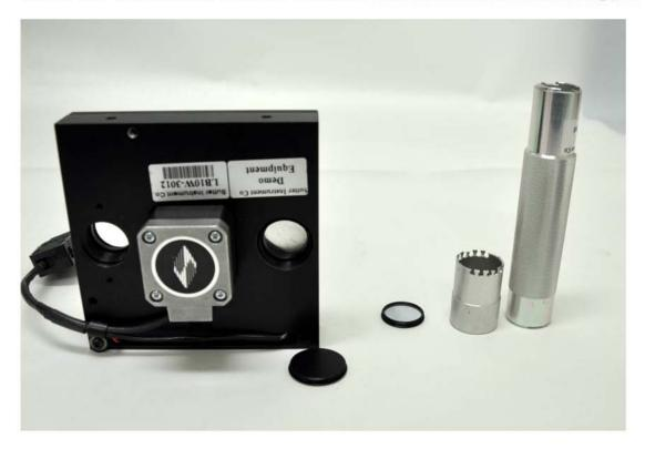
2. Use the cup side of the standard filter wrench to remove the cup from the filter wheel.
