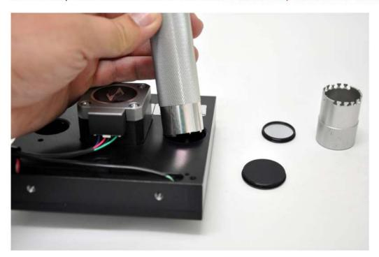
3. With the entire cup removed from the filter wheel you should visibly see the filter wheel itself through the loading port.
