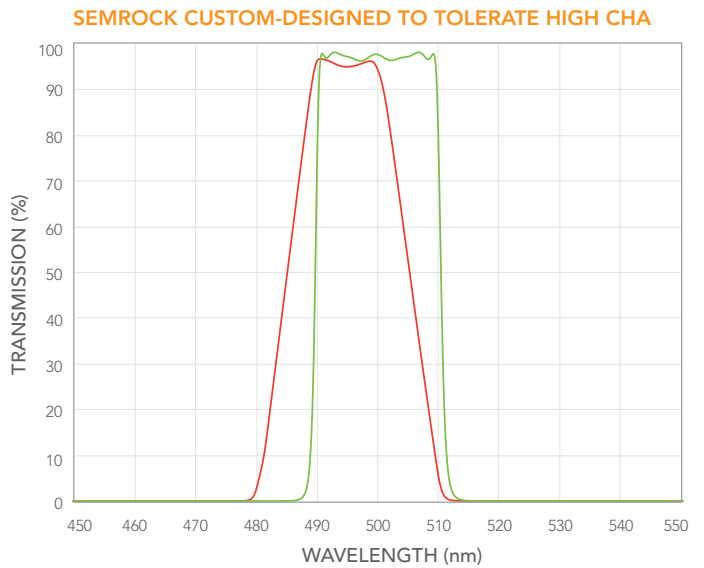
Figure 4: A standard filter without considerations to CHA shows reduced transmission performance, compared to a custom-designed filter with a high tolerance to high CHA. The green curve is CHA 0°. The red curve is CHA 25°.
