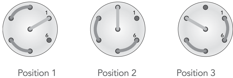
FIGURE 12. THE 3/7 INJECTOR WITH PURGE
