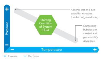
Any time system conditions shift in a way that reduces the gas solubility level of a fluid, outgassing occurs and bubbles form. If conditions change towards the lower right at any point in the fluid path, bubbles will be generated.
