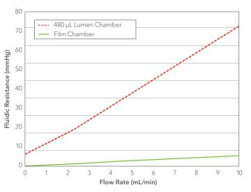
This shows the dramatic reduction in fluidic impedance, or fluidic resistance, with  $\rm H_2O$  at 27°C. There is ~0.1 PSI of resistance from 1 to 10 mL/min. This is about 5 mmHg pressure drop over the flow rate range.
