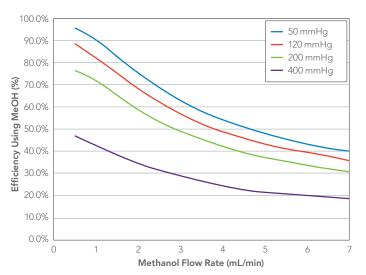
A characterization of the new IDEX Health & Science flat film degasser at various vacuum levels and flow rates produces a data set from which any particular performance curve can be derived. This data set allows complete control over the efficiency of the degasser, such that the degasser can be optimized for any flow rate within the vacuum range of the pump.
